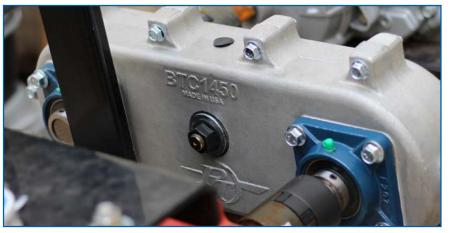
PT's BTC1450 Transfer Case has all moving parts contained and secured within the aluminum housing case. The internal belt is made of a premium-grade carbon fiber reinforced polypropylene.
